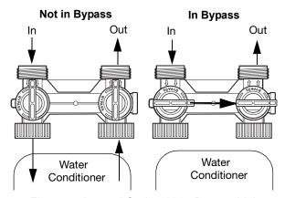
Figure 4 Autotrol Series 1265 Bypass Valve
