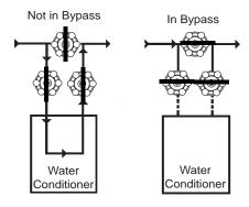
Figure 5 Typical Globe Valve Bypass System
